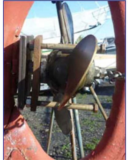
It worked. With pressure aft-ward on the propeller and shaft, the bolts holding the flexible coupling could be worked out of their holes and the parts separated.
